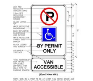
ACCESSIBLE PARKING SIGN DETAIL NTS
