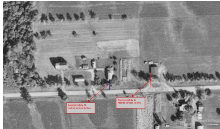
Figure 2: Aerial Imagery of the property from 1965, showing the existing barn to the east of the dwelling with red line showing 17 metres setback to front lot line. Blue line showing the 14 metres for the previous dwelling
